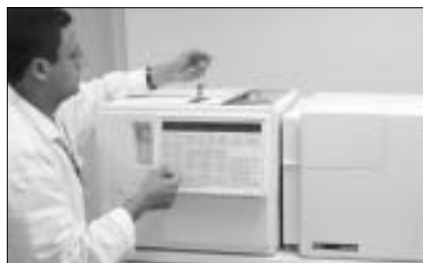
Samir Deshpande works at a Finnigan MAT GC-ion trap MS Magnum to analyze compounds.
