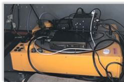
FINIS mounted in the aircraft on top of a mount to reduce vibration
