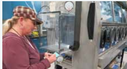
STC's Ms. Judy Castagno records pressure gauge readings on a glovebox used for conditioning systems under test.
